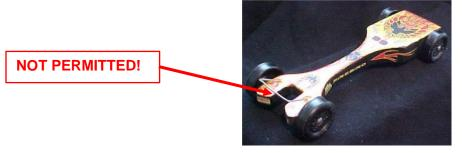
• The front of the car is to be and at least <u>1/2</u> inch wide where the car will make contact with the starting peg. Pointy nose cars such as Carrots, Arrows, Pencils, Rockets, etc... <u>ARE NOT PERMITTED</u> as the cars are difficult to stage and can create timing issues. Below are two examples of these types of cars.
